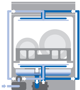
Tank system water intake
