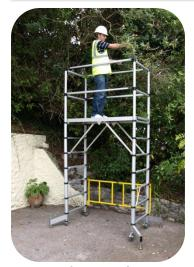
Can be used on uneven ground utilising stabiliser legs
