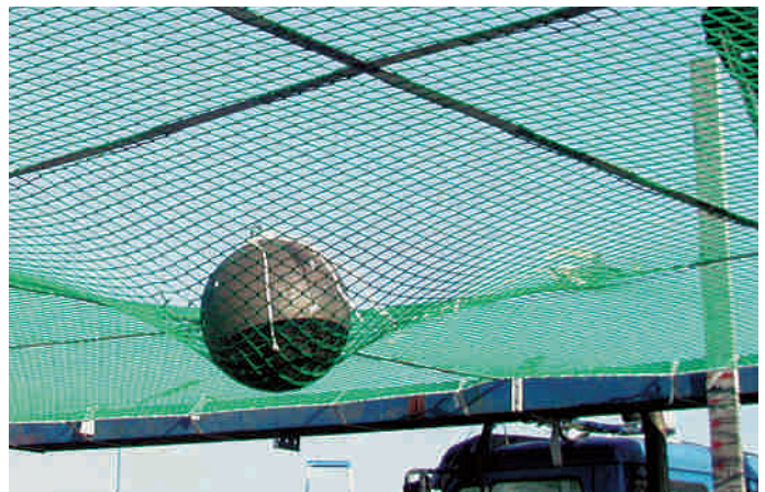
Test: the 100-kg iron ball was dropped onto the net from a height of 3 m.
