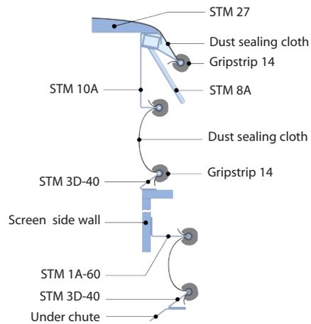
Picture 2. Section (typical) of dust sealed screen
