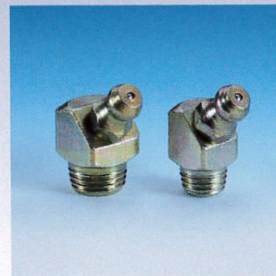
Lubrication Fittings with self-forming thread (180°-45°-90°) Form A, B, C according to DIN 71412 special hardened 650 HV
