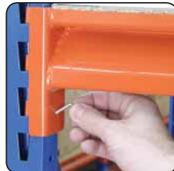
Secure location of beams
