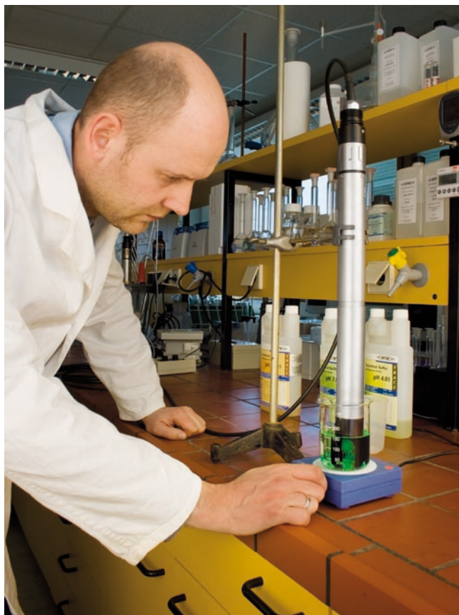
Laboratory pre-calibration of a digital sensor
