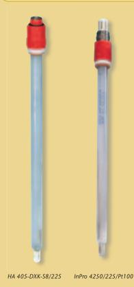
The InTrac® 777-SLM valve assemblies are fitted with combination pH electrodes with a XEROLYT® reference system. Using a polymer electrolyte, this system is superior to conventional design with gelor paste-type electrolytes with regard to operating reliability and working life. The twist-lock connector allows easy cable connection and simple electrode replacement.
