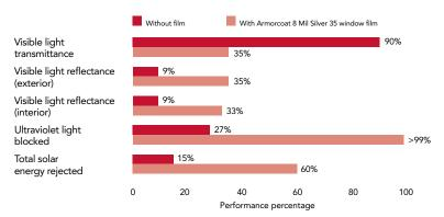
All performance results are based on the film installed on the inside surface of 4mm and 4mm+4mm thick, clear glass
