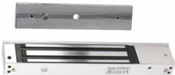
Electro-magnetical lock, mounted at the head of the door. Requires Z&L bracket for inward opening doors
