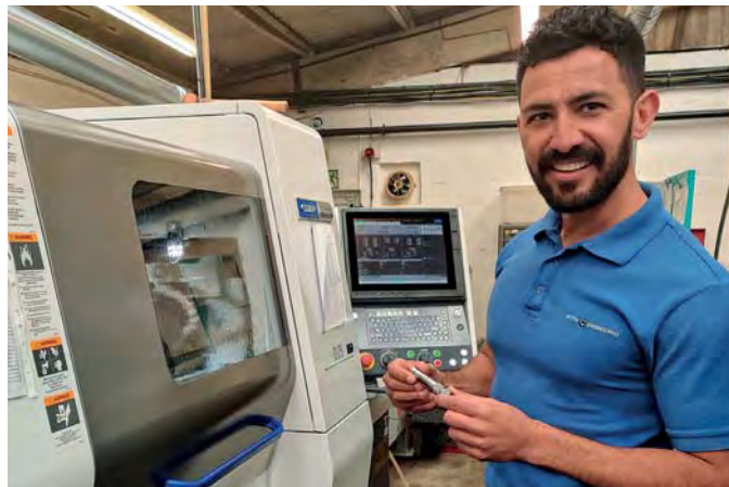
Machine operator Alexandre Da Silva in front of the Citizen Cincom D25-VIIIIFV sliding-head lathe on the shop floor in Barnstaple
