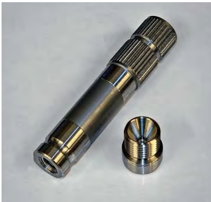
The lawnmower shaft (left) and a machined 304 stainless steel fuel inlet fitting, which was the second job to be put onto the D25
