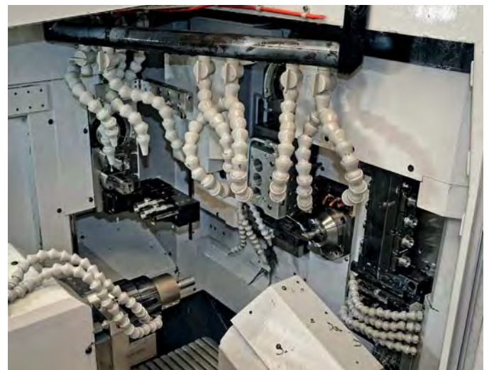
The working area of the D25, showing the twin-platen design
