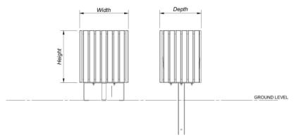
**Dimensions** Width - 390mm, depth - 340mm, height - 476mm excluding fixings (sizes are approximate)
