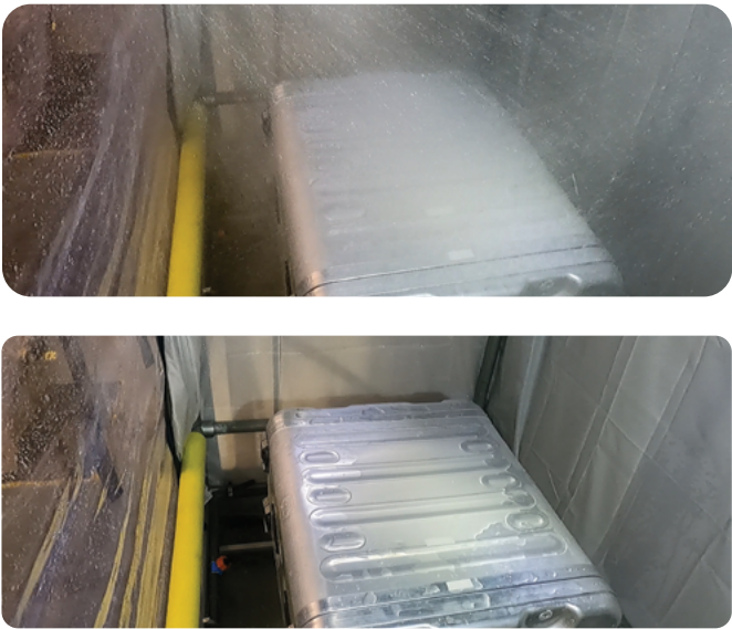
Water test rig delivering 300 Ltrs/min in conical and fantail jets
