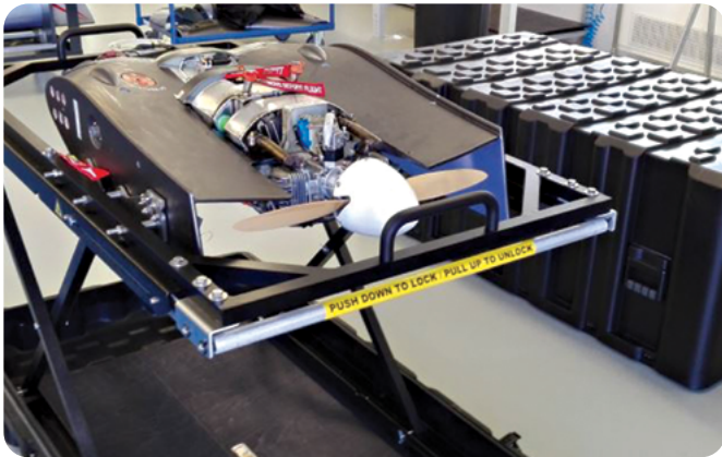
Rapid deployable Military UAV fuselage on a scissor jack platform – all inside an Amazon Container.
