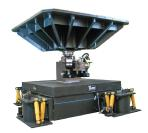
lbf. Our 80 Series actuators offer dynamic strokes up 12 inches and are available with a wide range of dynamic force outputs. Each vertical system includes our standard head expander and user defined insert pattern plus our air isolated, laminated steel reaction mass.
