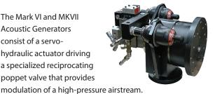
This design has proven to be the most effective sound source for large reverberant and progressive wave tube test chambers, providing extreme power handling capabilities with high efficiency. Peak acoustic pressures of approximately 60% of the supply pressure are produced downstream of the poppet valve.
