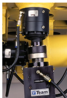
HydraBalls on both the MANTIS™ actuator and drive link.
