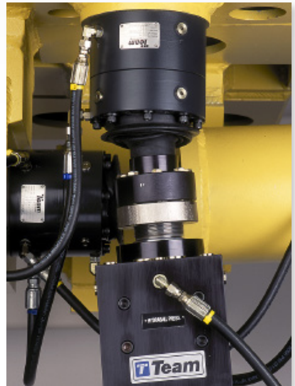
A pair of HydraBalls attached to a 6 DoF MAST table. The HydraBall in the foreground connects an actuator directly to the table, providing vertical excitation with compensation for lateral and longitudinal translations, as well as for any rotation.
