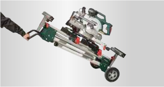
Trolley function for comfortable transport even with the saw mounted
