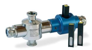
The Kemtrak DCP007 process analyzer is a high performance fiber optic coupled photometer for high resolution, real time, inline concentration and color measurement. Environmentally friendly, mercury-free LED light technology assures drift-free operation with exceptionally high precision.
