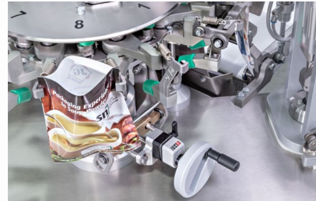
Central gripper adjustment (manual)
