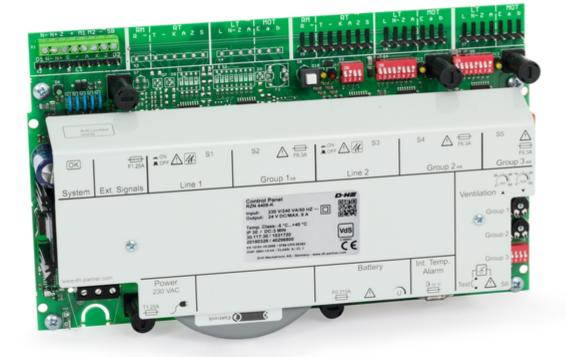
Improved voltage quality with plenty of power: The RZN 4408-K is one of the modular control panels and ensures the activation of SHEV and ventilation drives up to 8 A. AdComNet ready.
