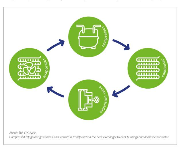
The technology has been used for over 100 years and is a proven and reliable method of removing heat from a space. By reversing this cycle, we can extract warmth from the outside air and use it to heat commercial buildings.
