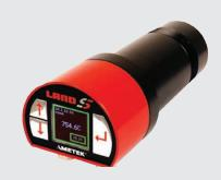
**TEMPERATURE RANGE** 200 - 1200 °C / 392 - 2192 °F An advanced non-contact infrared spot pyrometer specifically designed for continuous, highly accurate measurement of coated steel strip temperature during galvanising and galvannealing.
