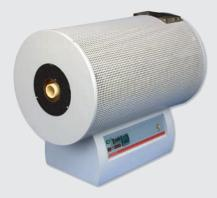
A comprehensive range of blackbody primary and reference sources providing high-precision calibration of radiation thermometers under on-site or laboratory conditions.
