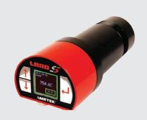
**TEMPERATURE RANGE** 600 - 1800 °C / 1112 - 3272 °F An advanced non-contact infrared spot pyrometer specifically designed for liquid metal temperature measurements in foundry and tapping applications..
