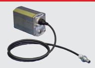
**TEMPERATURE RANGE** 800 - 2600°C / 1500 - 4700°F A short-wavelength infrared thermometer providing precise and stable temperature measurement for control of optical fibre drawing tower furnaces.
