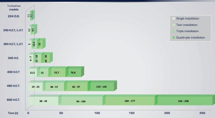
The maximum suggested displacement is purely indicative as this depends on hull shape, LCG, installed power etc... Please contact Castoldi for advice on any application.
