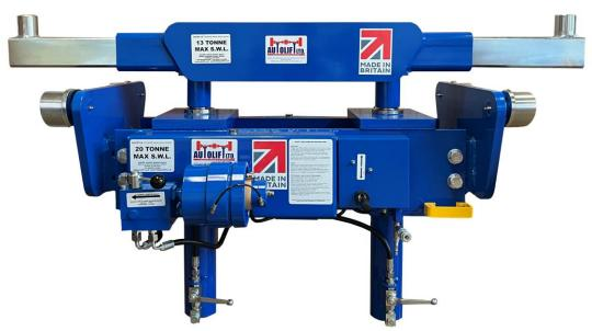
Pit must be a minimum of 900mm wide for rams to be able to spread far enough apart to fit the 13T Telescopic Spreader Beam on. Lifting points range from 920mm to 1400mm.
