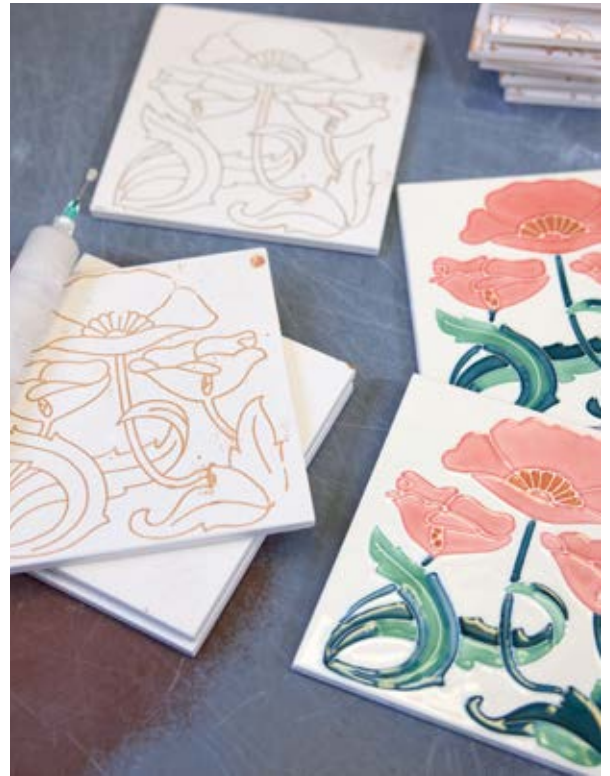
▲ Tube lined tiles before and after decorating
