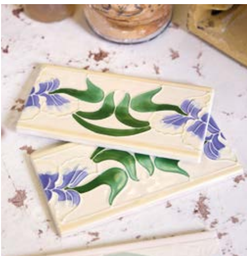
▲ Once the tiles are fired the glazes are rich and translucent
