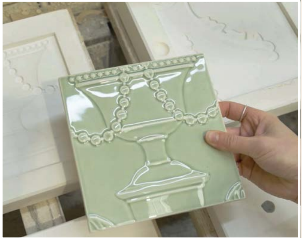
▲ Bespoke glazed moulding with plaster moulds
