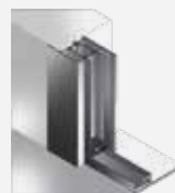
E: Installation in-between daylight opening using an interior cover strip
