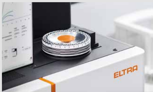
Detachable sample carousel for high sample throughput
