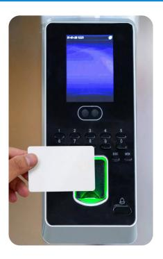
Access control is a system that allows you to manage who can enter or exit certain areas of your property. This type of security system uses various methods of identification tools to allow access to a specific area.
