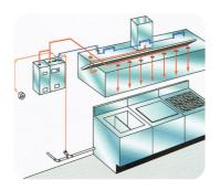
A kitchen system consists of ductwork and a suppression unit.
