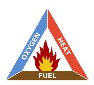
elements are heat, oxygen and fuel. The simplest elements to remove are heat and oxygen. For example a water jet fire extinguisher works by using the cooling effect of the water to remove the heat from the triangle, whereas a CO2 extinguisher removes the oxygen. A foam extinguisher aims to remove both, with the foam acting as a cooling agent but also a barrier to prevent further oxygen from reaching the fuel source.
