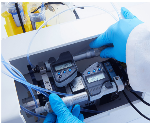
Figure 2: LyobeadPro Instrument - Adjusting the Dispensing Volume.
