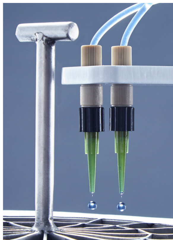
Figure 1: LyobeadPro instrument - Droplets during dispensing prior to freezing.
