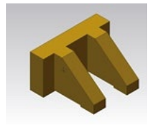
GB = Gusset Back: having a fin on one side that is not attached to the belt but rests on it and increases rigidity when the cleat is pushed in one direction
