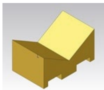
CR = Cradle Shape: "U" or "V" shaped so that an object can rest in the seat created by the sides of the cleat
