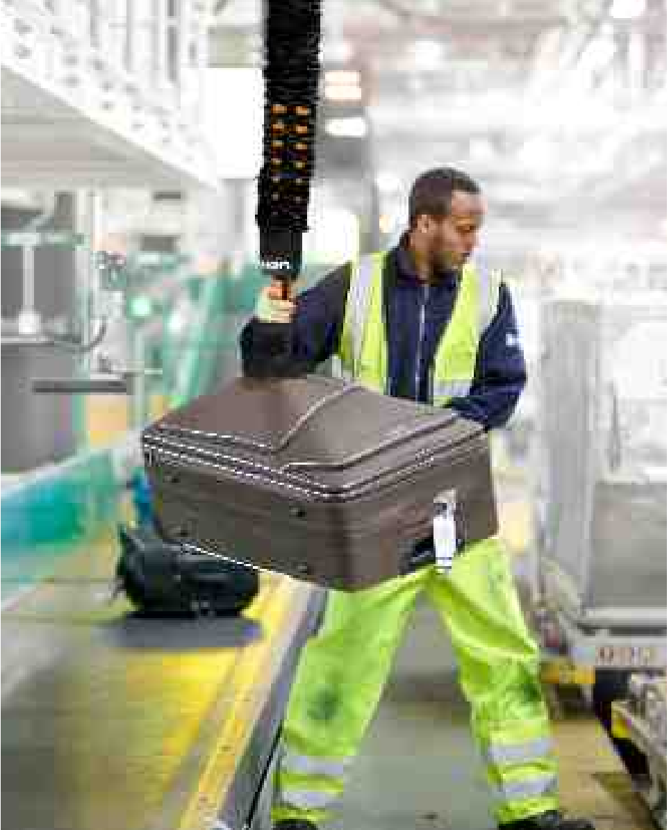
Heavy baggage handling is easy and effortless with our high frequency vacuum lifter. The baggage can be rotated 360 degrees before it is placed and the angle adapter allows the operator to angle the suction foot at 90 degrees to pick up bags from the side.
