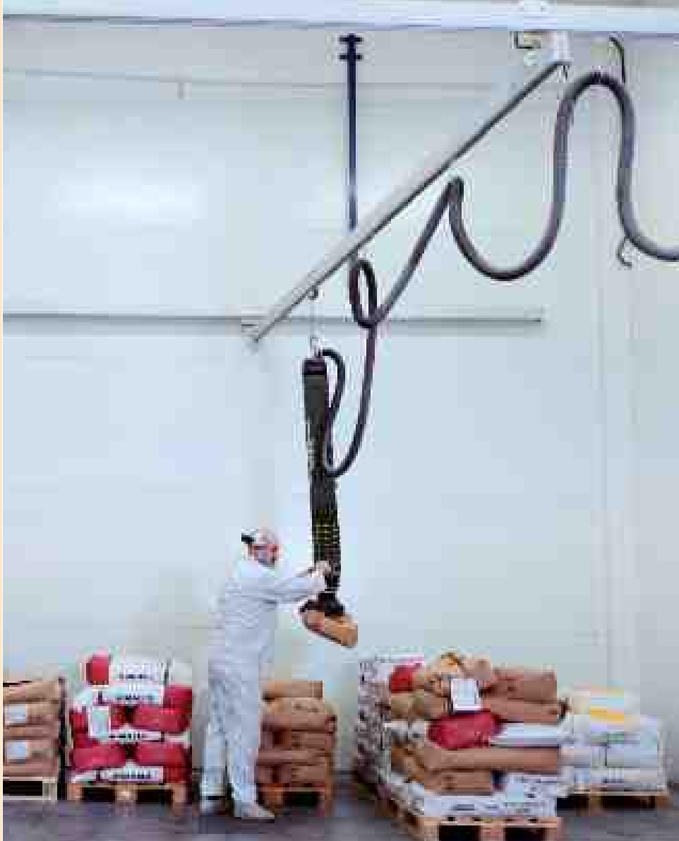
Stable trolleys run smoothly in the profiles, steadily moving your lifter to where you need it.
