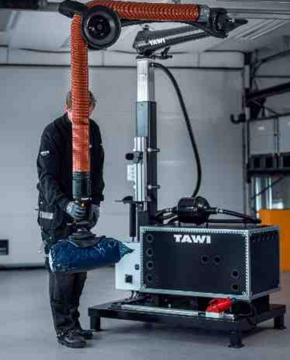
The mobile high frequency lifter can reduce two-person lifts to one and be split across contracts to reduce labour.
