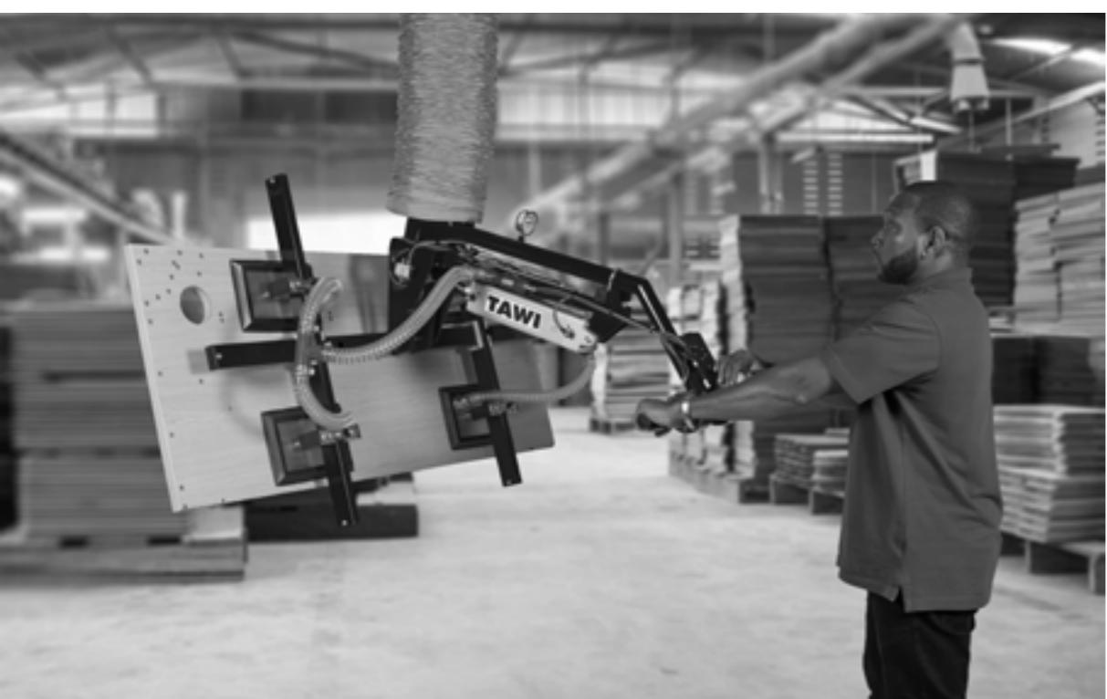
Lifting, moving and placing large wooden sheets with our panel lifter is safe and reliable.
