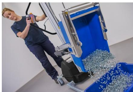
Ergonomic handle for easy and comfortable operation. The lifter is belt driven which ensures quiet and smooth oil free drive.
