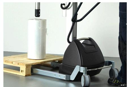
On several models, the measures of the wheels make it possible to drive the lifter into a Euro-pallet in three different ways.
