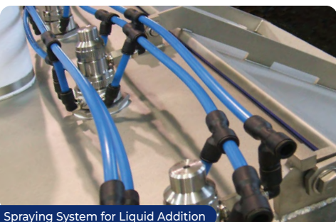
Spraying System for Liquid Addition
