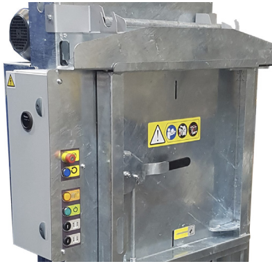
Galvanised finish Corrosion-resistant coating for outdoor or harsh, wet environments.
