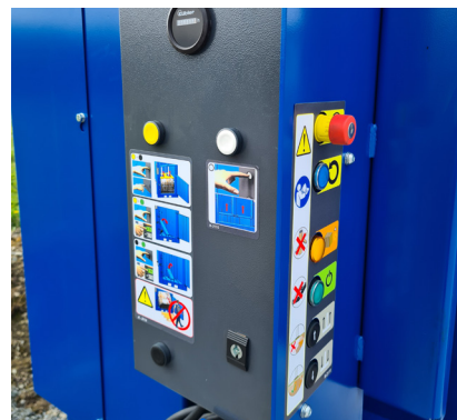
Auto PLC control panel with bale full light Includes automatic compaction cycle, bale full indicator, E-stop, and key-lock control.
