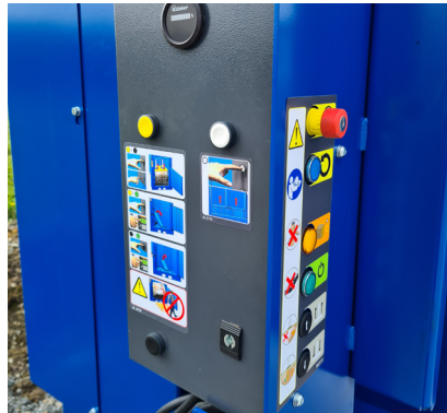
Auto PLC Control Panel Includes automatic compaction cycle, E-stop, and key-lock control.
