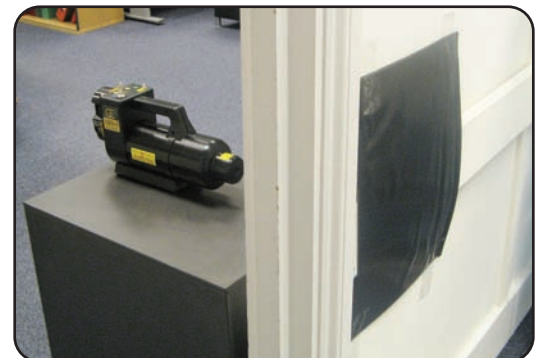
Flexible image plate taped to a wall for room search or counter surveillance work
