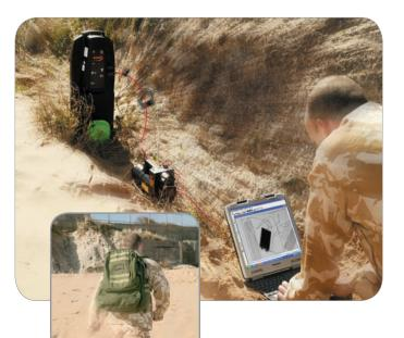
Developed specifically for portable x-ray screening in tough law enforcement and EOD environments, Scanwedge has a unique flat panel design which allows it to be used in even the most confined spaces. Scanwedge can be used from different orientations and produces high quality x-ray images.
