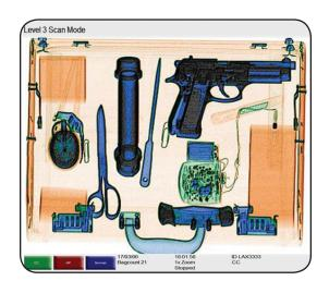
The Rapiscan 618 is a high performance converorised x-ray scanner designed for customers requiring a compact and portable x-ray machine with a fast throughput of mail and bags.
