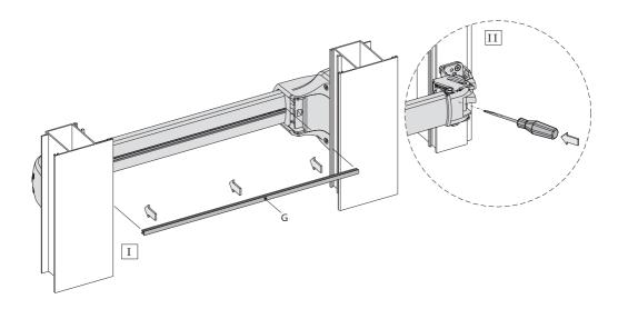
For the fitting of the "**G**" garnish (optional; to be used only for aesthetical reasons) see fig. I, starting from the ends. In case of removal, operate with a 3mm screw driver, as shown on fig.II.
