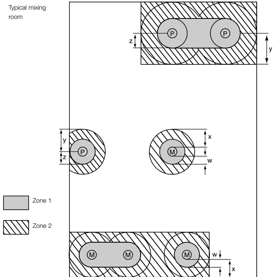
M = mixing vessel P = pump
