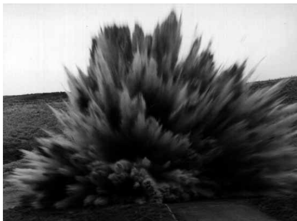
Figure 3 Musk xylene detonation following initiation by 200 g of high explosive
