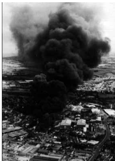
Figure 2 In 1992 a major fire in a warehouse demonstrated the consequences of accidentally overheating a stored energetic substance. 2 The incident was made worse because the substance was also stored with incompatible substances. In that incident an energetic substance was stored too close to a steam heating pipe. The heat from the pipe caused the substance to decompose with the result that the drum burst and the substance was spread around the store. The substance settled on an oxidising agent stored in the same room and the resulting mixture ignited. The ensuing fire destroyed the warehouse
