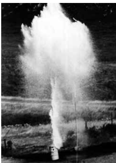
Figure 4 Alcohol wetted nitrocellulose undergoing a deflagration following an initiation by a pyrotechnic device
