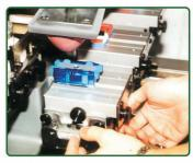
2 individual X,Y angle platform/work table with independent adjustment
