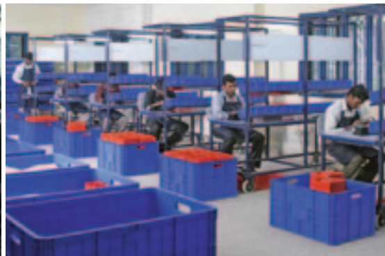
Assembly of audible and visual signalling devices (brand Clifford + Snell) in Chennai, IN
