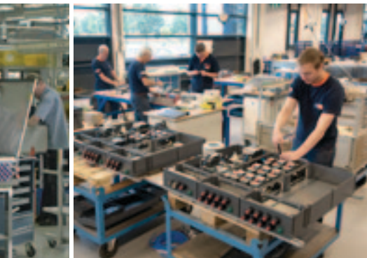
Assembly of distribution panels (series 8146) in Hengelo, NL
