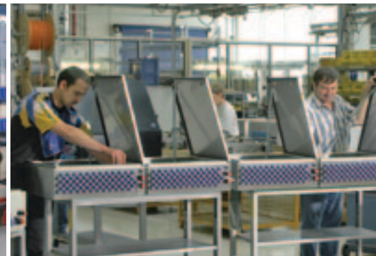
Assembly of switch cabinets in Waldenburg, D
