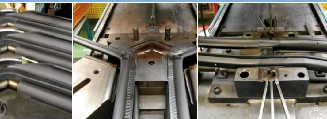
Vulcanisation around corner
