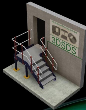
Fire Escape Staircases.
