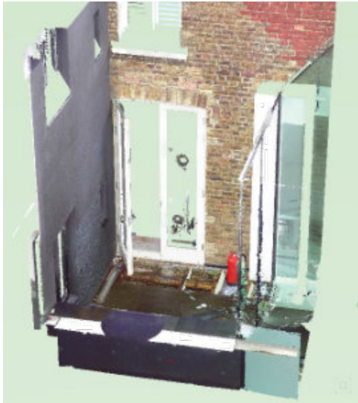
A point cloud produced by our laser scanner.
