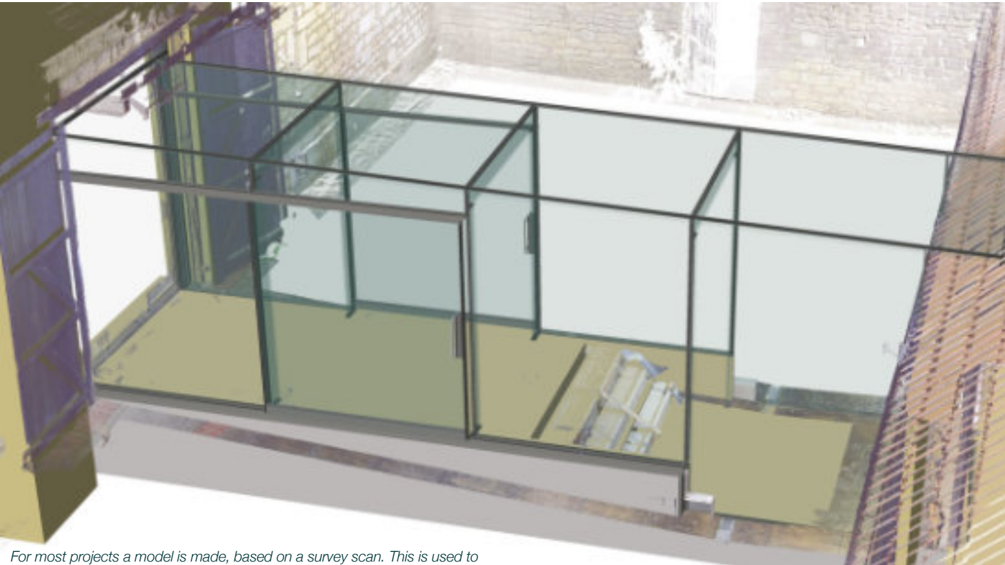
For most projects a model is made, based on a survey scan. This is used to evaluate and refine the design. The model can then be used to produce planing and production drawings
