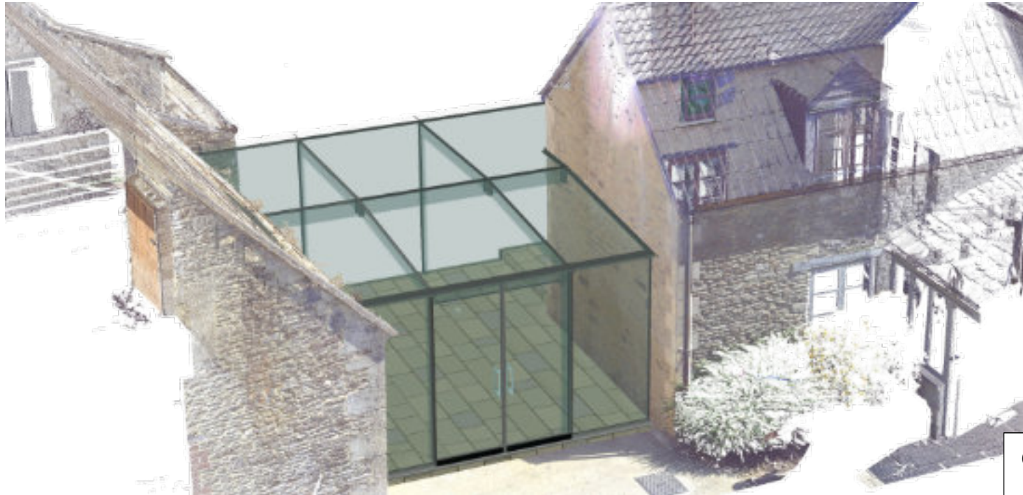
A point cloud with proposal added. Buildings, especially old buildings are often not square or regular. Glass can be cut to fit the irregular form of a building closely.
