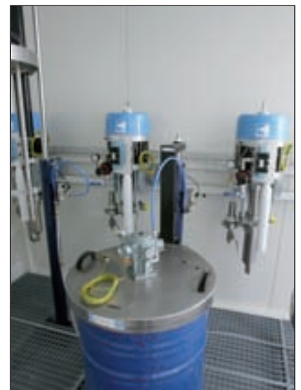
Figure on the right: The flexible interior can be adapted to your individual requirements. In this case, several agitators and dosing stations have been installed.
